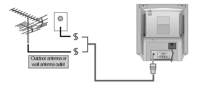
If TV picture is not clear, it usually result from the wrong antenna connection. Please install the antenna in the proper place and in the right direction.
